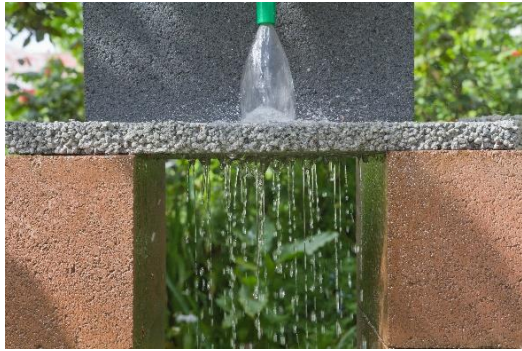
Permeable (Porous) Pavement Example
